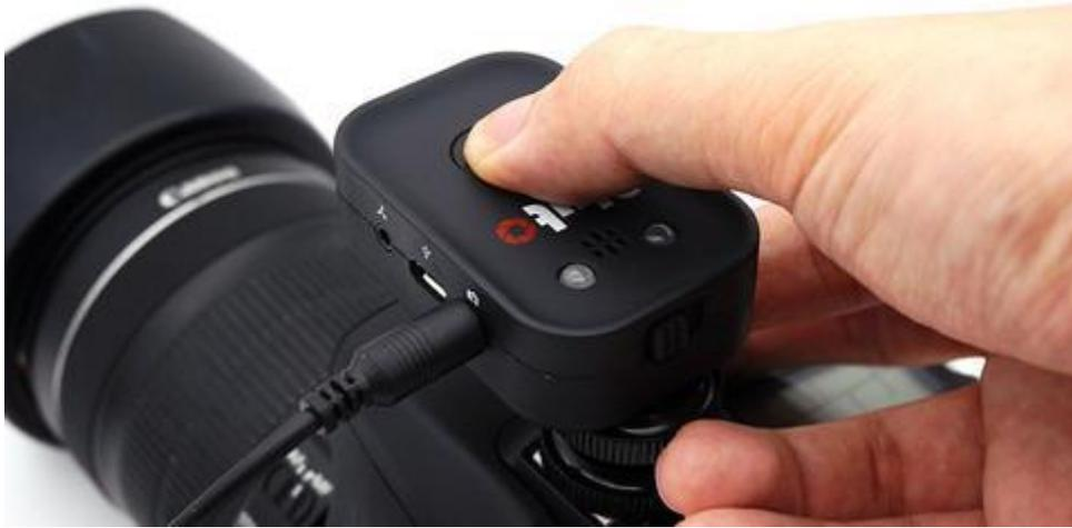
If the app found your Pluto Trigger in the last step, move on to the next step. Otherwise, try turning on your Pluto Trigger's Bluetooth. Press and hold the button on Pluto Trigger for at least 5 seconds. If the status LED blinks three times, then Bluetooth has been turned on. If the status LED blinks only once, then Bluetooth has been turned off. Press and hold again to turn Bluetooth on.
