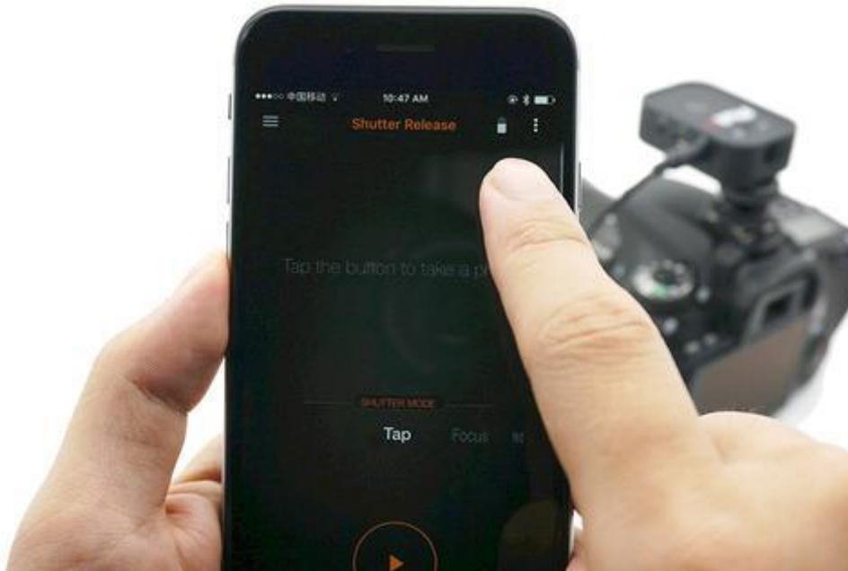
Once connected, the Pluto Trigger's blue LED will blink once. The app will make a notification sound. Navigate back to the main screen. The spinner will have been replaced by a battery icon. This battery icon indicates the remaining battery on your Pluto Trigger.
