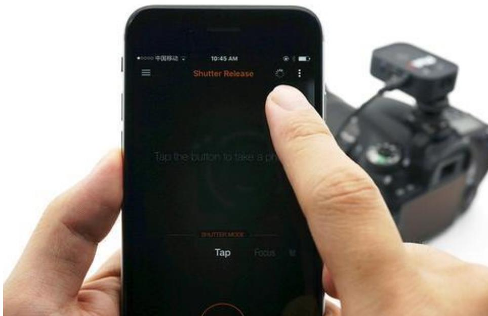
For your first use, you will need to pair your app with your Pluto Trigger according to the following steps. Later on, the app will connect to your Pluto Trigger automatically. **Do not pair using iOS or Android's Bluetooth settings, it will be rejected.**
