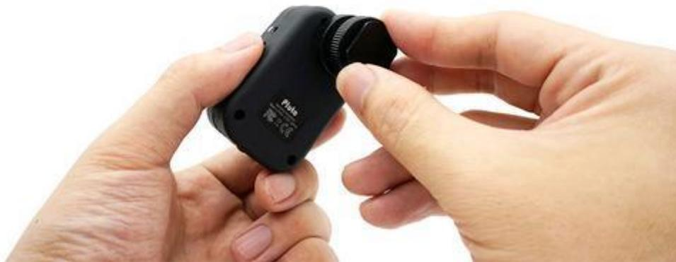
Screw the hot shoe adapter into Pluto Trigger.
