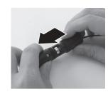
3 Place the new battery, with the + and - oriented as indicated, into the battery compartment in the power pack. The + symbol is stamped inside the compartment for reference.
