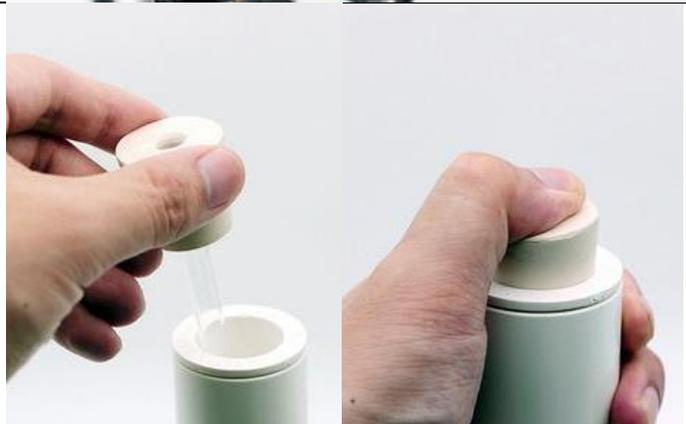
Insert and press the small tube. Make sure the air above the water and between the small tube and the big tube does not leak.
