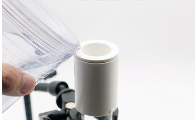
Fill the tube with water so that the water level covers the bottom of the small tube. Never let the water level go below the bottom of the small tube, or else the valve will not be able to keep constant pressure.
