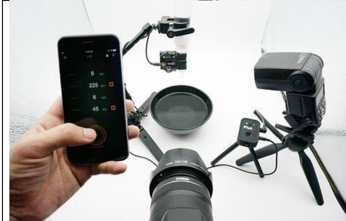
Turn on your Pluto Trigger. Launch the Pluto Trigger app on your phone. Set the IR settings to match your camera model. Select Droplet mode from the menu. Press the start button to test. The Pluto Trigger should send IR commands to trigger your camera, release two droplets and then trigger your flash.
