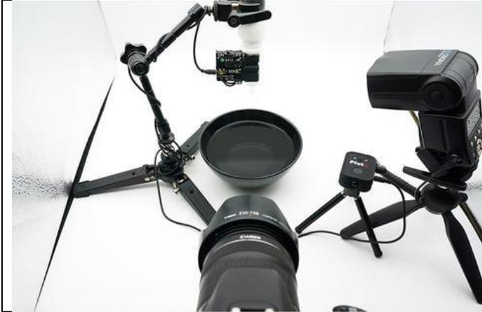
Water droplet collision photos need to be taken in a almost dark room. You will need a camera, a speedlite flash, a tripod, and a magic arm to hold the valve and the Pluto Valve Kit.
